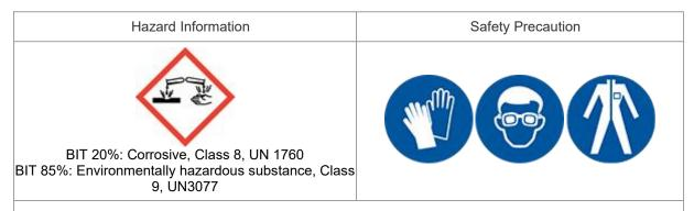
The operation must be carried out in strict accordance with the regulations. Avoid contact with skin. Wear protective clothing, goggles and rubber gloves. In case of contact with skin, wash immediately with plenty of water and soap. If splashed into eyes, wash immediately with plenty of water and buffer..
